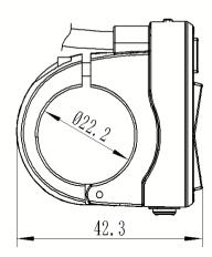
Open the controller clamping jaw and place it on handlebars in your chosen position. Use an Allen wrench to tighten the locking screw M3x8. Tightening torque: 1 Nm
