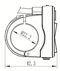
Open the controller clamping jaw and place it on handlebars in your chosen position. Use an Allen wrench to tighten the locking screw M3x8. Tightening torque: 1 Nm
