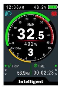
Battery indicator of capacity (48,2V at illustration image)
