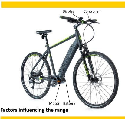
**1.** Rolling resistance of the tyres. Leader Fox e-bikes are fittet with tyres with low rolling resistance and increased resistance to puncture. It is also important that the tyres are inflated properly. Therefor, if the tyres of your electric bicycle are underinflated, the range will decrease.
