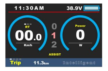
RT Speed -indicator of speed mode(RT, MAX, AVG)
