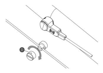
Tighten the nut D by a flat screwdriver.
